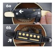
**STEP 6a**: with the strings still removed, turn the pickup upside down and prepare for soundhole installation. The wire coming from the pickup should be on the treble side of a standard right-handed guitar. Move the left side spring clip to a 45 degree angle (6a).
