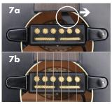
**STEP 7**: on the right side of the pickup, rotate the spring clip so the bent section is visible. Place the pickup in a centered and level position within the soundhole, then rotate the round button arm (7a) of the spring clip to the right and out of sight (7b). This will place the right hand spring clip in place to securely hold the pickup in the soundhole.
