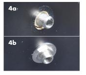
**STEP 4**: with guitar strings removed, reach inside the guitar's body to insert the jack from inside the guitar towards the outside of the end block through the 15/32'' hole (4a). While holding the jack in place, install the washer and hex nut to the smaller threaded area on the outside of the guitar. Finger tighten the hex nut (4b).
